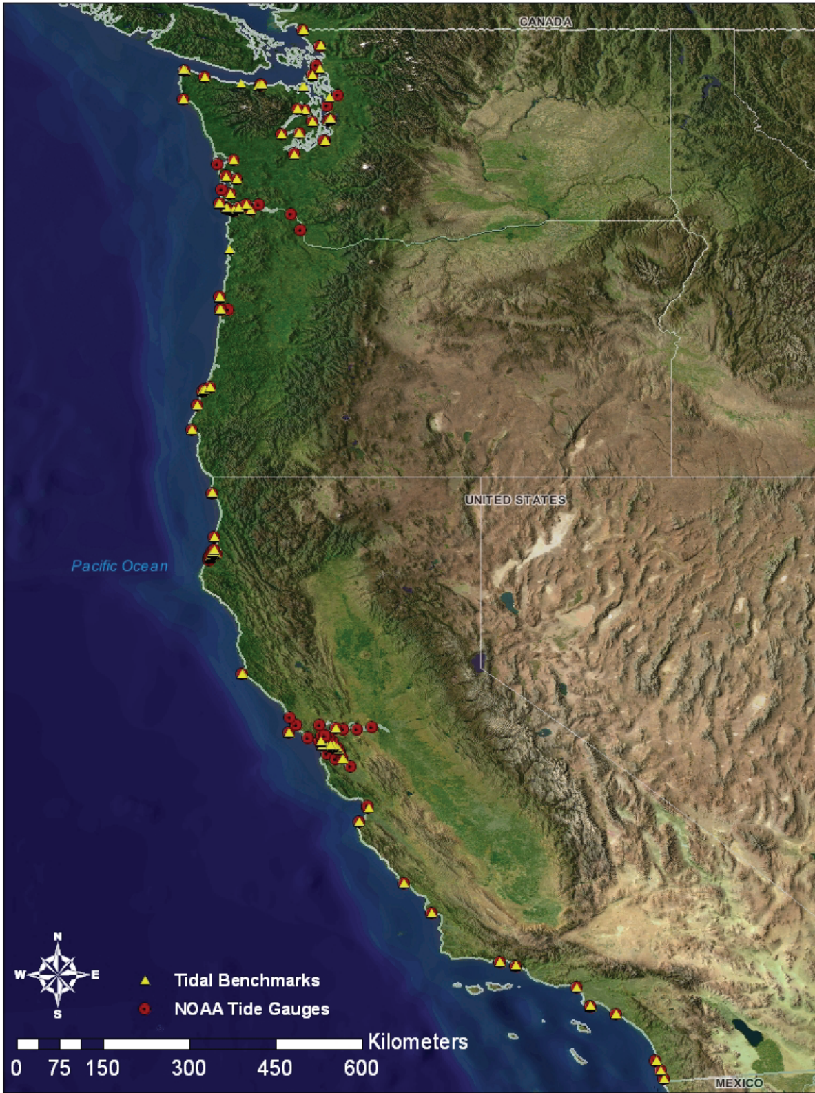
Figure 15. Location of tidal benchmarks and tide stations used to compute the West Coast of the Continental United States VDatum TSS grids.
