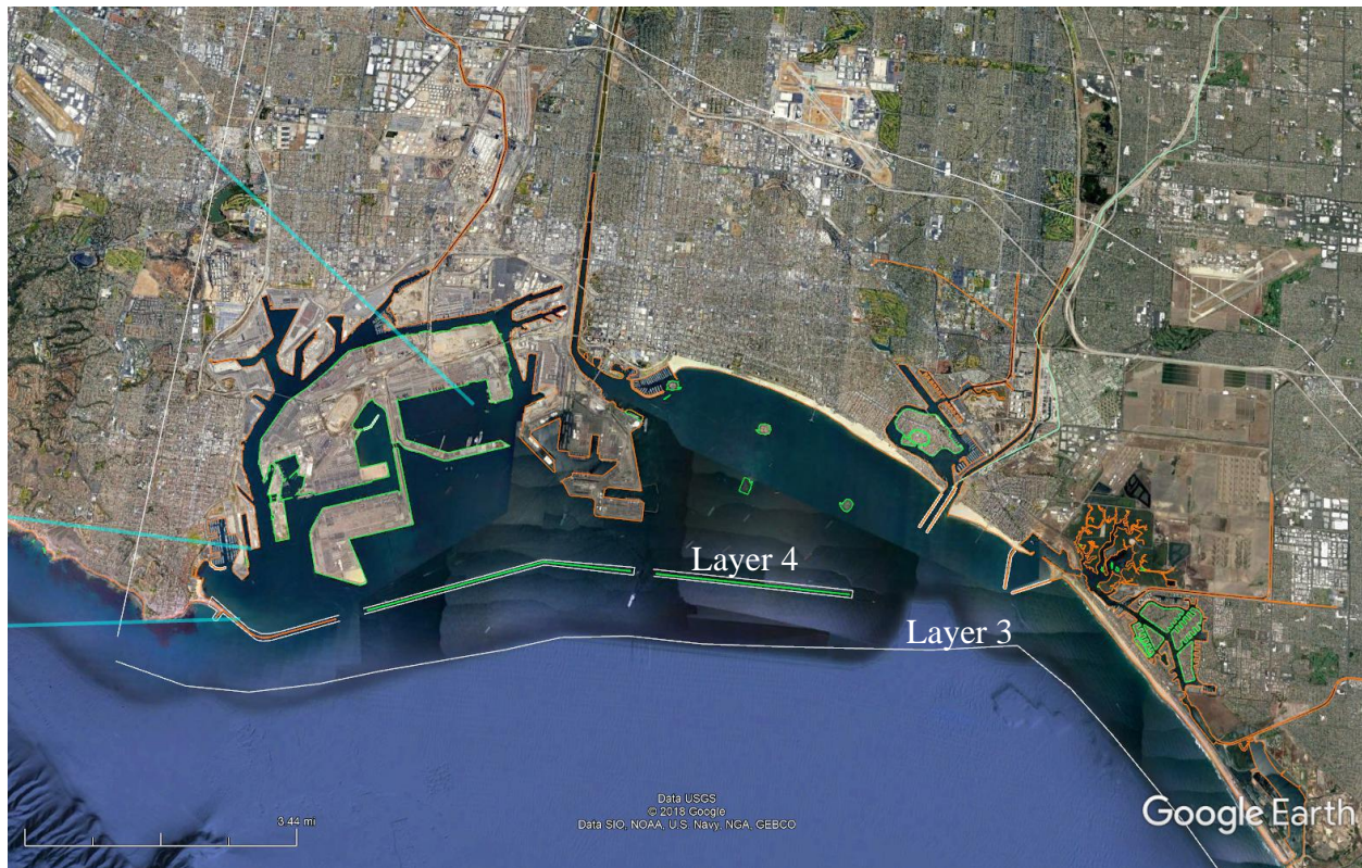
Figure 11 Examples of OceanMesh 2D Layers 3 and 4 in Los Angeles. White, the one Layer 3 polygon for the Harbor and 9 Layer 4 polygons for breakwaters and jetties. Green, island shoreline; Orange, mainland shoreline.
